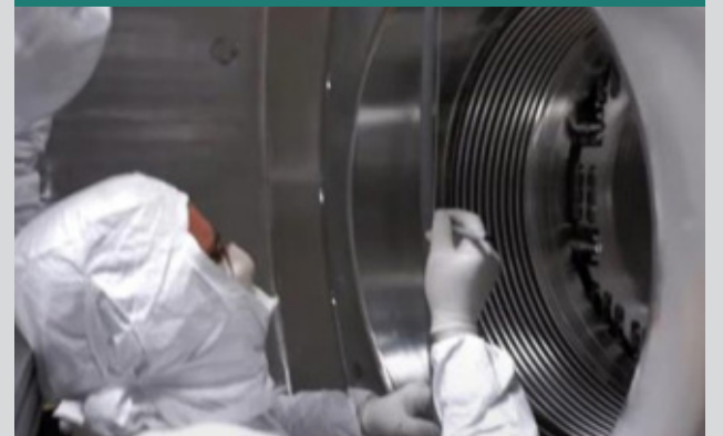
Oval, rectangular & circular multi-ply bellows for the Wendelstein 7-X Stellarator, Germany
