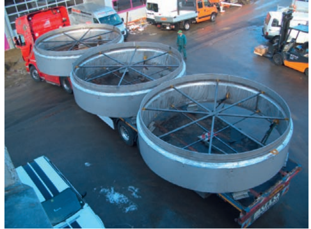
Gasturbinen Kompensatoren DN 4300 Gas turbine expansion joints DN 4300
