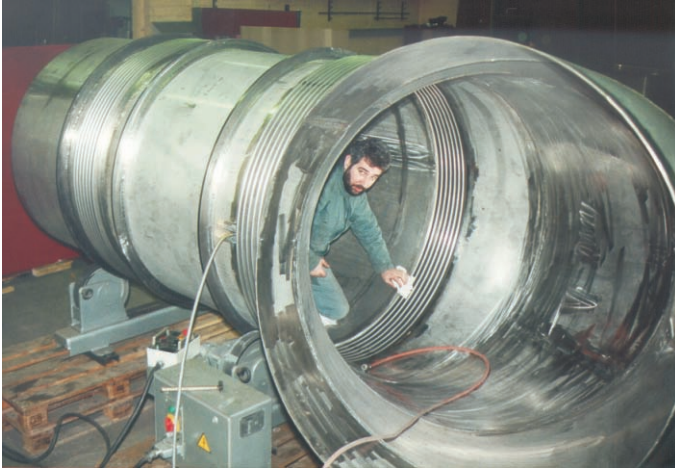
Eckentlasteter Chromstahlkompensator Corner balanced expansion joint
